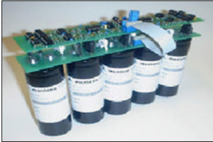
Figure 10. Super capacitors assembled in series [28]
