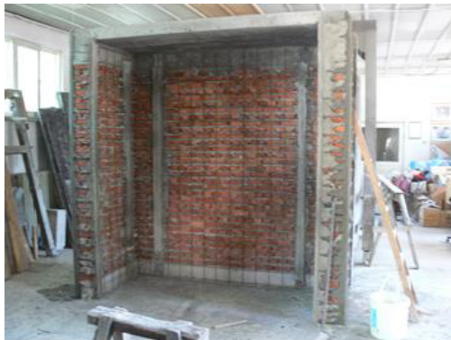
Figure 12. Inner wall covering with steel mesh (Ateş, T.)
