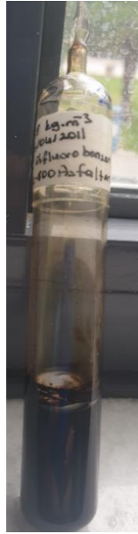
Figure 2: The sample in Pyrex tube was sealed and degassed.
