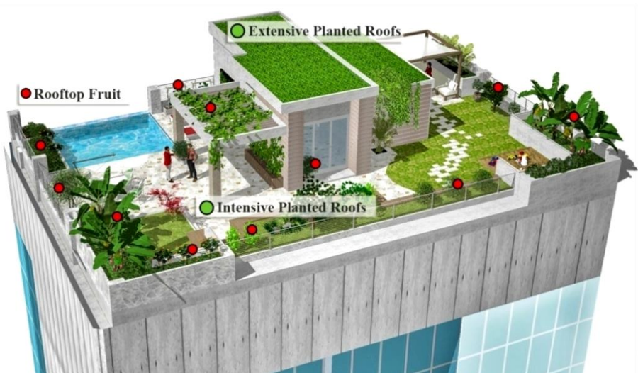
Figure 4: Roof Garden with an Example of Extensive and Intensive Type and the Use of Fruit Species (Original by Grubač)
