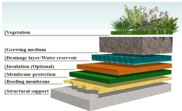
Figure 2: Typical Cross Section of a Green Roof System (Original by Grubač)
