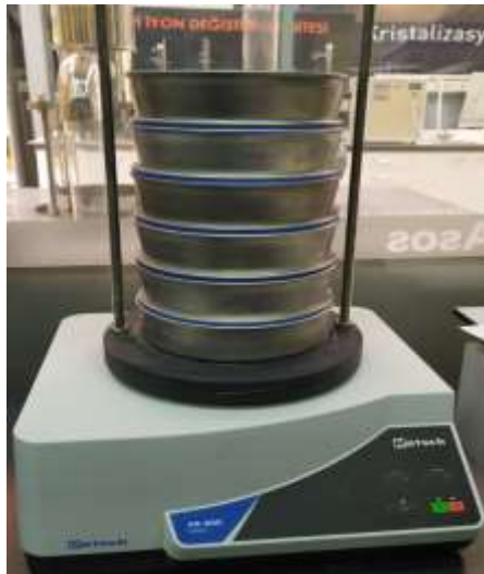
Figure 3. Reetcsh As 200 Basic sieve device
