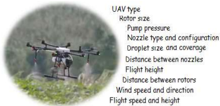
Figure 1. Equipment-Related Factors Affecting Application Success in Pesticide Applications with Unmanned Aerial Vehicles
