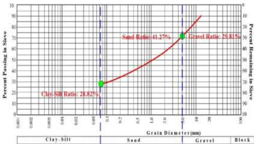
Figure 15. Grain size distribution graph of the impermeable layer
