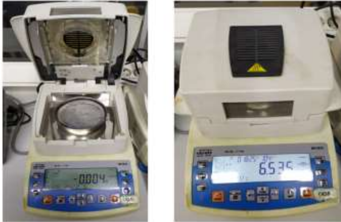
Figure 2. Radwag MA50.R moisture analyzer
