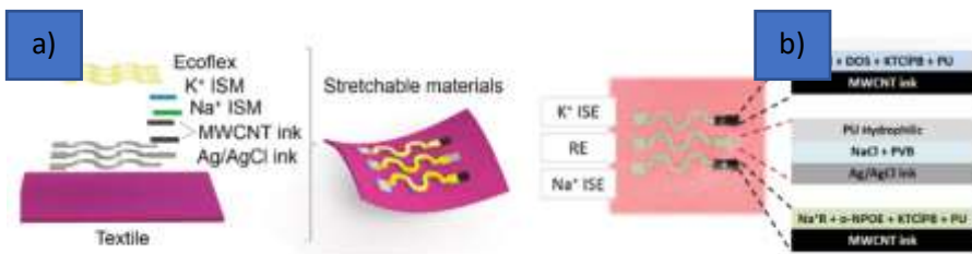
Figure 2. a) Manufacturing processes and materials of stretchable materials; b) image of ion-selective membranes. Reproduced from (Parrilla et al. 2016)
