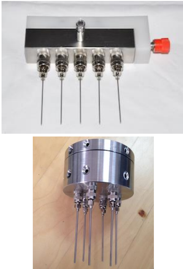
Figure 2. Linear multi-needle and multi-coaxial electrospinning spinneret
