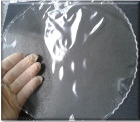
Figure 4. Optimized bioplastic prepared using myofibrillar proteins from gilded catfish (Araújo et al., 2018).
