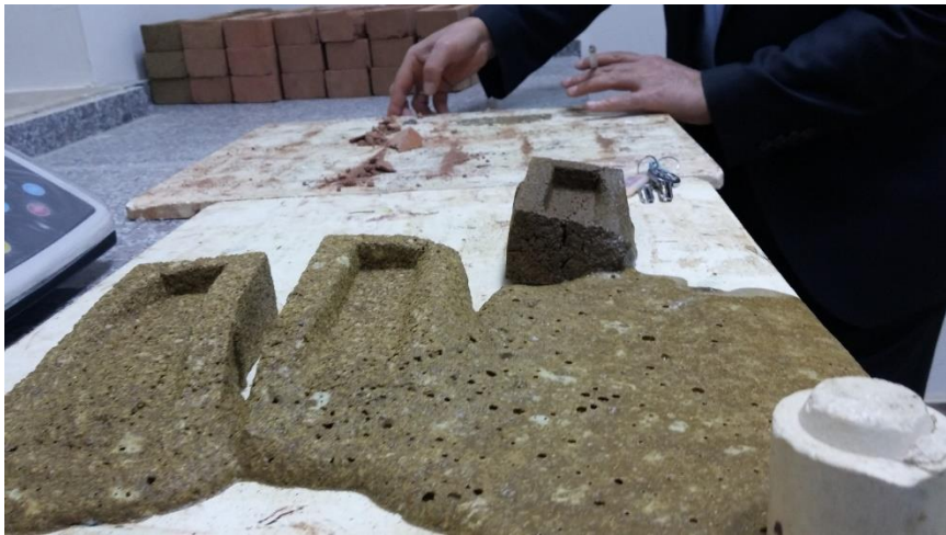
Fig. 13. Conversion Of Brick Samples To Liquid Phase At 1200 °C
