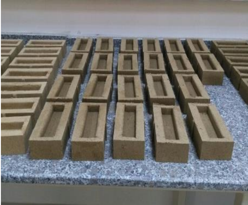
Figure 2. Bricks produced in the dimensions of 15 cm x 7 cm x 4 cm
