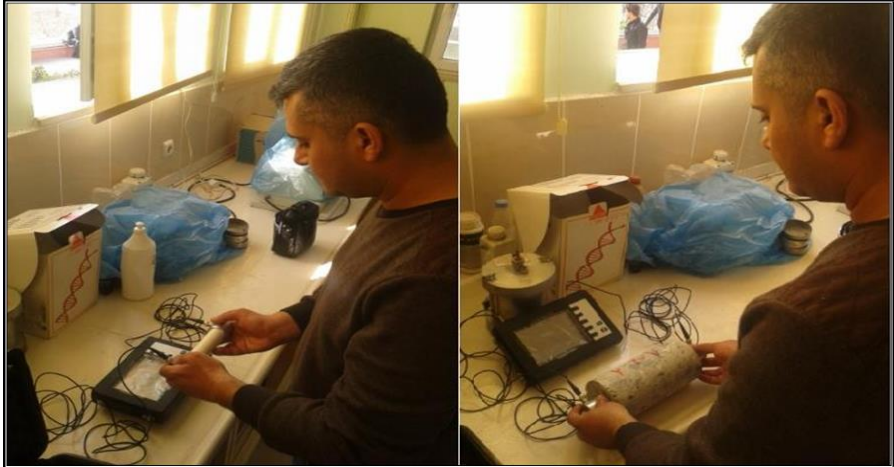
Figure 7. Calibration of Ultrasound Device and Ultrasound Test Applied to Samples
