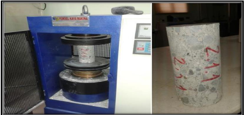
Figure 8. Pressure Test Applied to Core Samples
