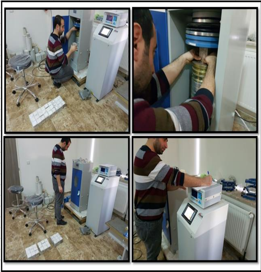
Figure 3. Concrete that has been hardened and measured for compressive strength
