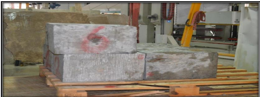
Figure 3. Concrete Samples Cut To 40x40x25 cm Dimensions
