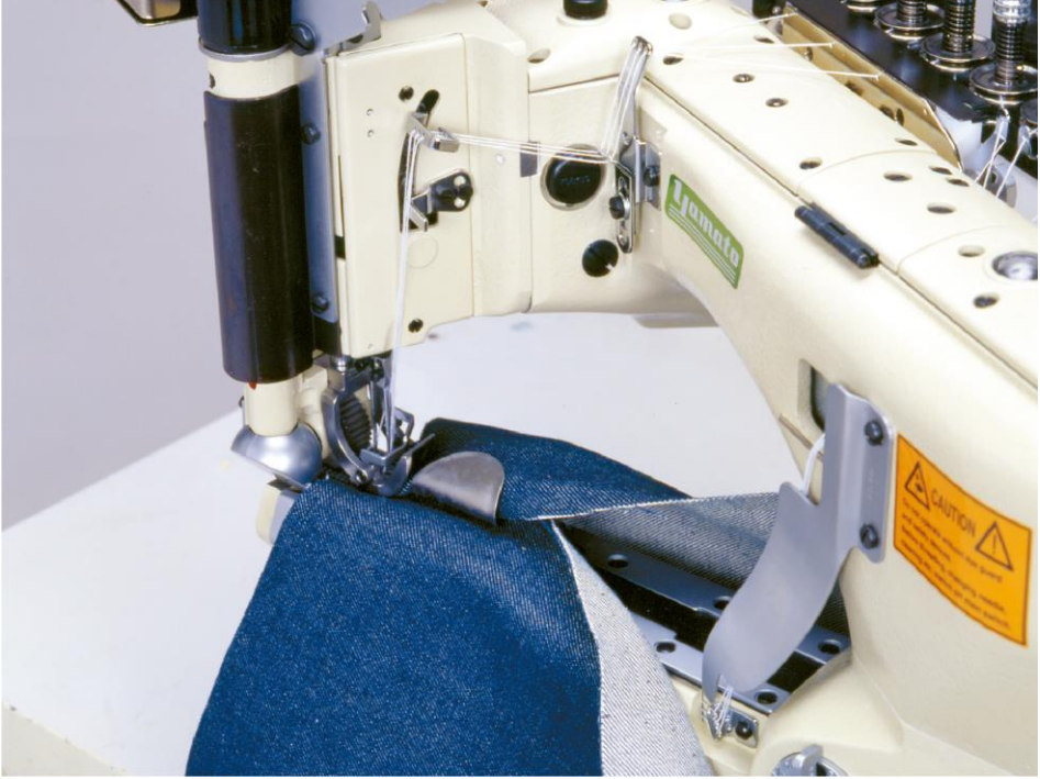
Şekil 84. Kollu kot makinesi ( https://www.yamato-sewing.com )
