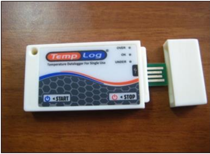
Figure 1: Templog-ig150 data recorder used to store internal temperature values in the trials
