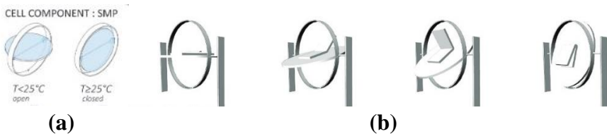
Figure 9. SMP Baseline Cell Prototype (a) Open-closed position according to temperature; (b) Adaptive movement in the simulation model (Yoon, 2019)
