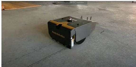
Figure 32. Printer Robot can draw one-to-one with the project (Badré, 2020).
