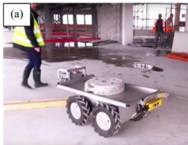
Figure 30. Autonomous Rover will follow workers carrying heavy items (Hassan, 2018)
