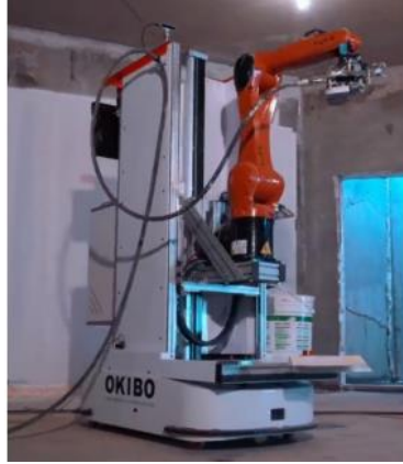
Figure 23. Painting robot developed for interior of buildings (Khadka, 2021).
