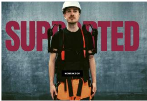
Figure 25. Wearable robot supporting worker (Bock et al., 2012)
