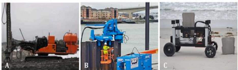
Figure 31. Sheet piles driving robot examples (Melenbrink et al., 2020).
