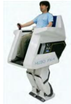
Figure 25. Wearable robot supporting worker (Bock et al., 2012)
