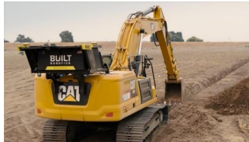
Figure 29. The truck which the software is installed performs autonomous excavations. (Melenbrink et al., 2020).
