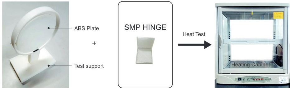
Figure 10. SMP Baseline Cell Prototype Components and Heat Test Setup (Yoon, 2019)
