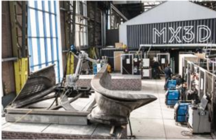
Figure 11. A steel bridge is made as 3D printing (Melenbrink et al., 2020).
