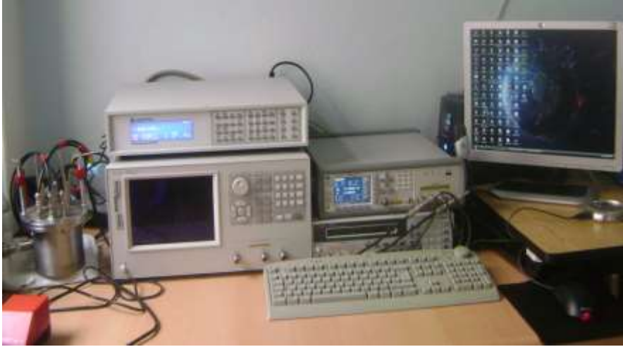
Figure 13. Dielectric Meter Device (Agilent E4980A Precision LCR Meter) (Şahin, 2010)
