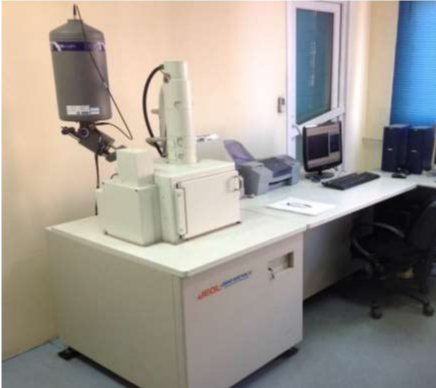
Figure 26. A Picture of the SEM (JEOL 5910-LV) Setup in the Testing Room for the Material with EDS (Oxford-Inca-7274) (Şahin, 2019; Şahin, 2010)
