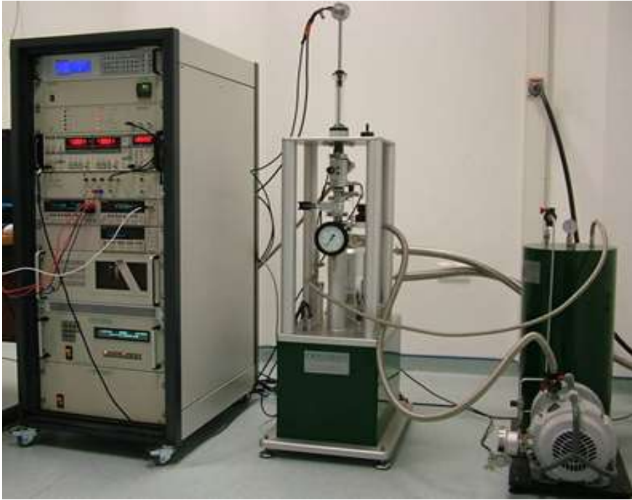
Figure 7. Cryogenic Limited PPMS Device for VSM (merlab.metu.edu.tr) (Şahin, 2019)
