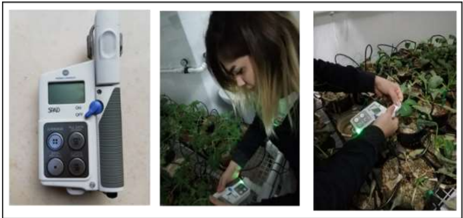
Figure 15. Measuring Plant Leaves with A Portable Chlorophyll Meter (Savcı and Deveci, 2022)
