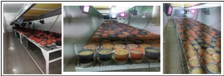
Figure 4. Plastic Pots With A Volume of 800 ml (13x11cm) on the Growing Tables in the Climate Chamber (Savci and Deveci, 2022)
