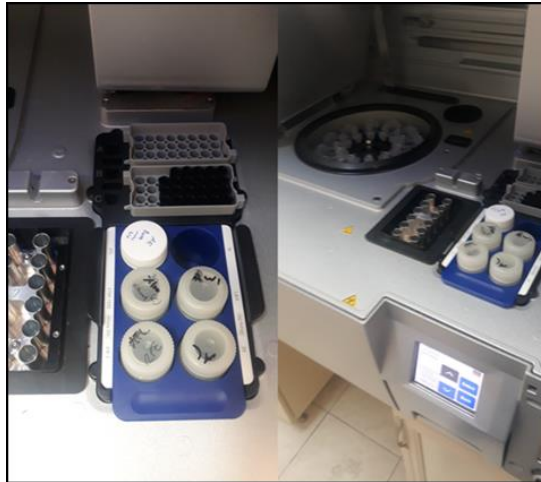
Figure 4. The parts where the QIACUBE automatic isolation robot and buffers are placed.
