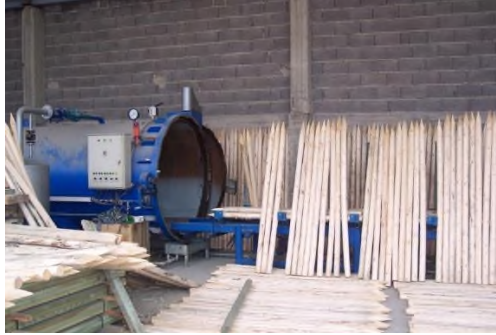
Figure 1. A Pressurized Impregnation Facility Applying The Vacuum-Pressure Method (Bozkurt, 2009).
