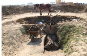
d. Kneading Mud e. Transporting the mud from the pond f. Brick mold
