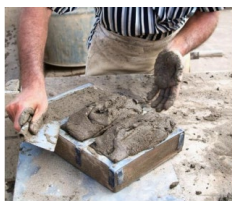
g. Sanding of molds h. mud pressing into the mold i. Arranging the bricks in the drying area
