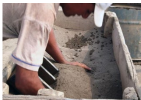
g. Sanding of molds h. mud pressing into the mold i. Arranging the bricks in the drying area
