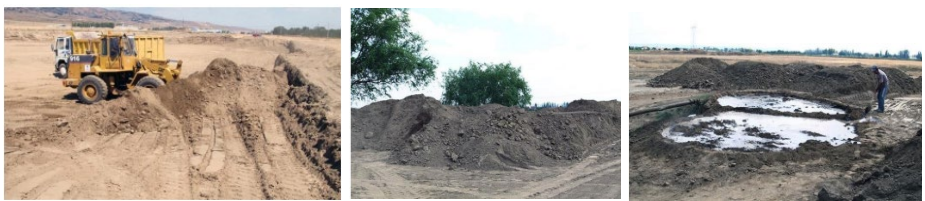
Figure 1a. Transport of raw material b. Brick soil c. Preparation of sludge in the mud pond
