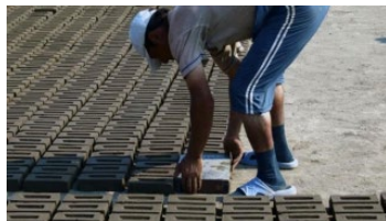
g. Sanding of molds h. mud pressing into the mold i. Arranging the bricks in the drying area
