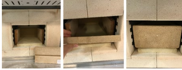
Figure 6. Refractory bricks were placed on inner surfaces to ensure equal heating in the furnace.
