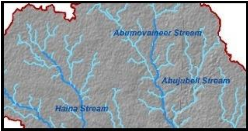
Figure 25. Dendritic (Tree) Drainage Model which is the Most Common Drainage Type in the Study Area
