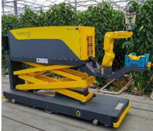
Figure 8. Project of SWEEPER, a sweet pepper harvesting robot prototype (Arad et al., 2020)
