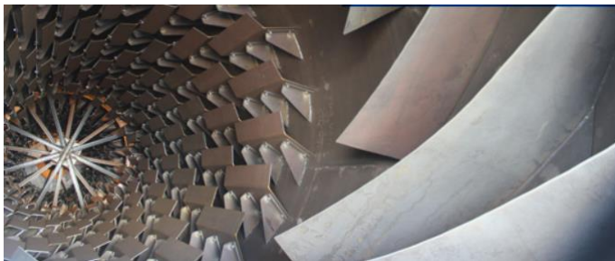
Figure 8. Optimal drum interior design for fertiliser quality (Feeco, 2023)
