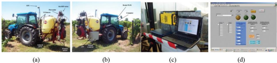
Figure 7. (a) and (b) Placement of components on the sprayer, (c) laptop for wireless control of the prototype from the tractor cab, (d) interface for input data created using LabVIEW (Gil et al., 2013)
