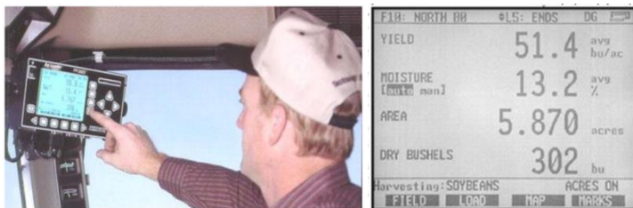
Figure 2. A yield indicator placed inside the harvester cabin (Keskin et al., 2000)
