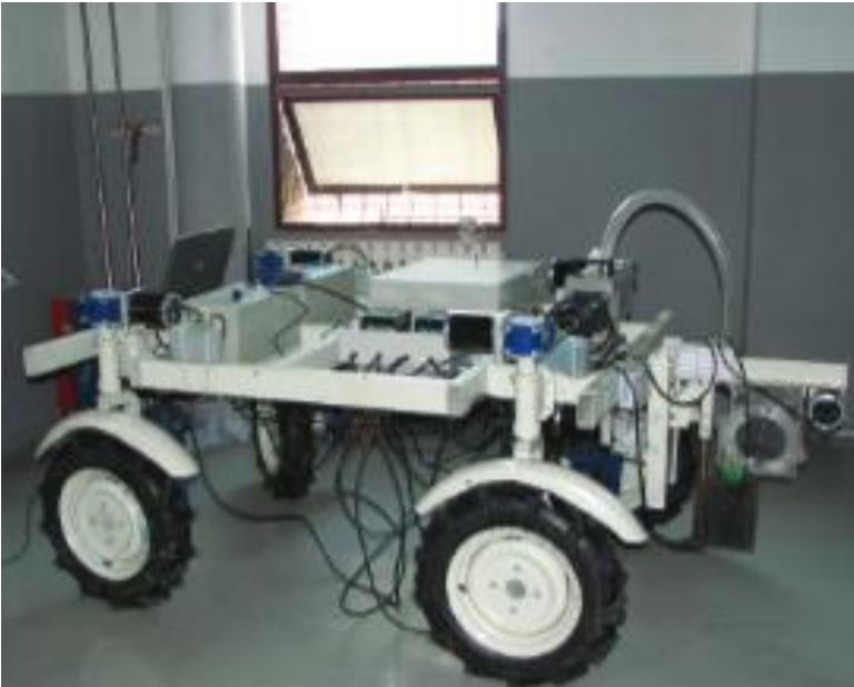
Figure 5. Wheat precision seeding robot (Lin et al., 2015)
