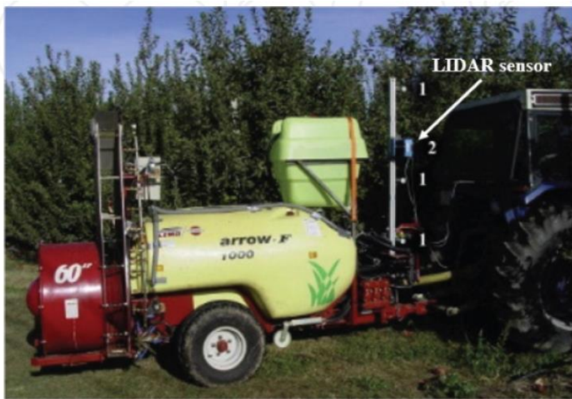
Figure 12. Variable-rate orchard sprayer prototype implemented with LIDAR sensor (Escolà et al., 2013)
