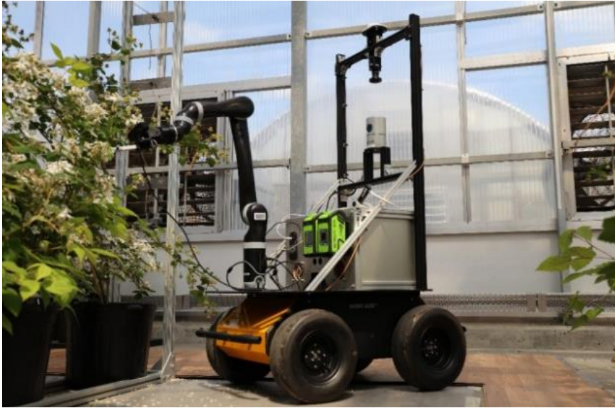
Figure 6. Precision pollination developed by Virginia University (Ohi et al., 2018)
