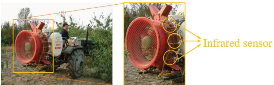
Figure 2. An automatic target-detecting air assisted sprayer working in orchard (He et al., 2011)
