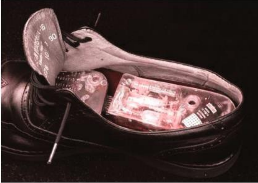
Figure 5. The first modern concept of a wearable device invented by Thorp and Shannon (Guler et al., 2016)
