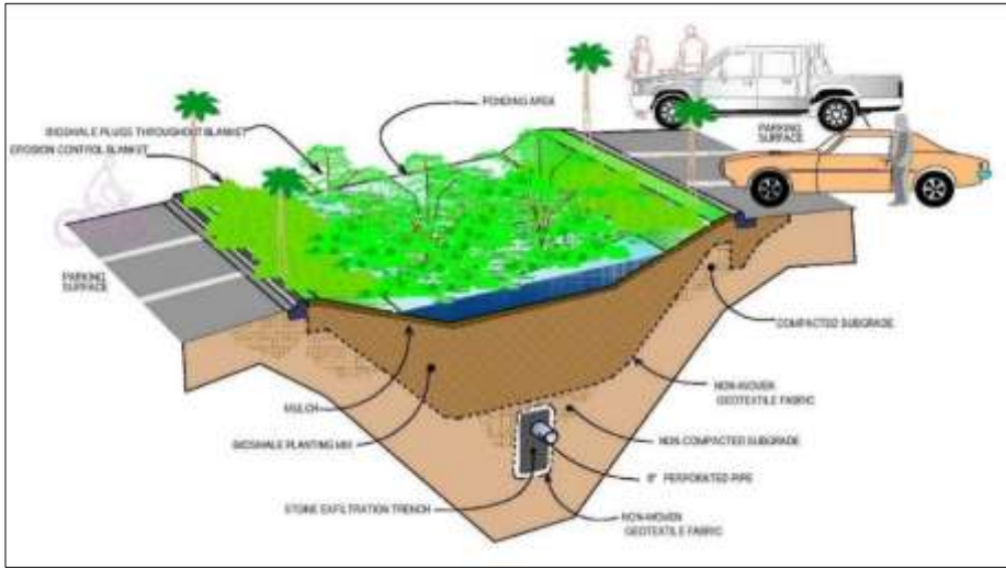
Figure 12. Bioswale concept diagram, structure and operation (Faraj and Hamaamin, 2023).
