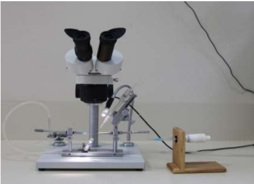
Figure 1. Instrumental Insemination Unit
