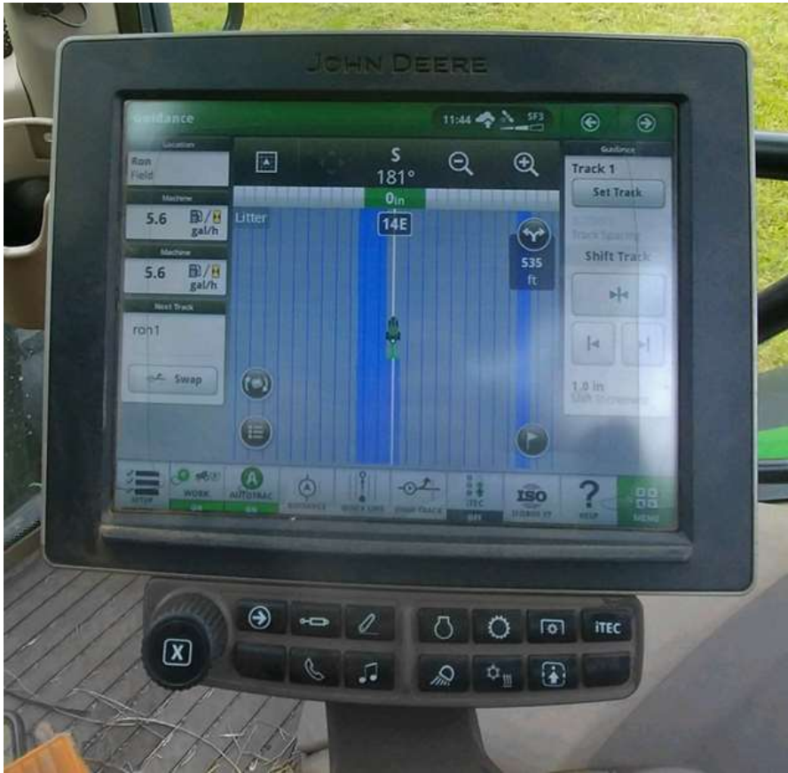
The tractor-guidance screen as seen during a fertilizer application; the blue lines are the areas covered by the tractor. Photo by Dr. Mike Popp, University of Arkansas
