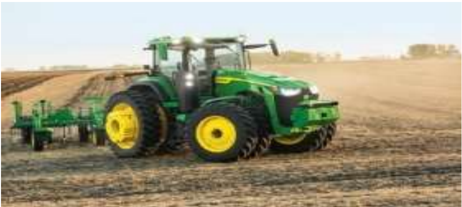
Figure 1 John Deere autonomous tractor navigates crops without a driver
