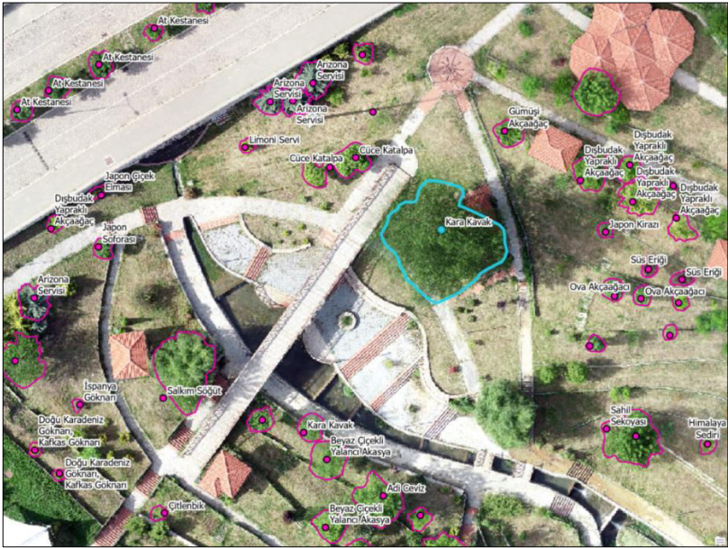
Figure 3. On-screen digitization method based on the orthophoto map of the Seyitler Campus. Tree positions (red dots), crown projection areas (red boundaries), and name tags (local species names in Turkish) are displayed on the GIS database. The turquoise-colored boundary highlights the crown of the largest tree, Populus nigra .
