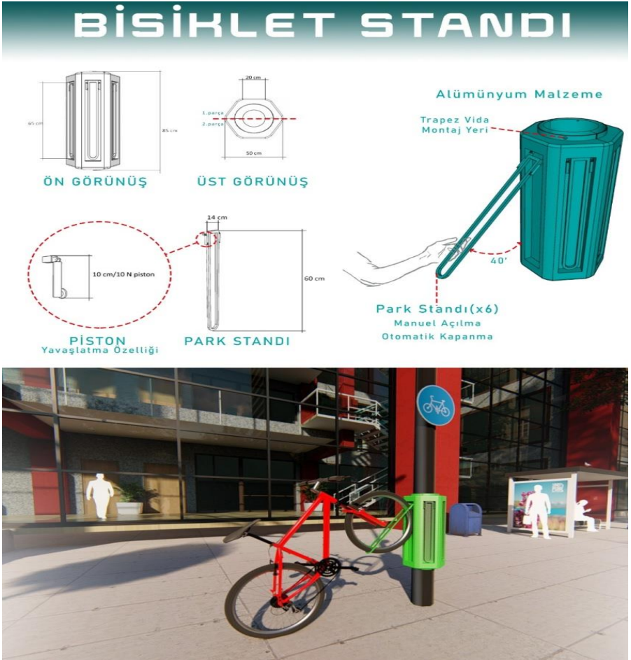
Figure 9. Computer-Aided Design of a Tekno Bicycle Stand with Specification and Detailing (Original)
