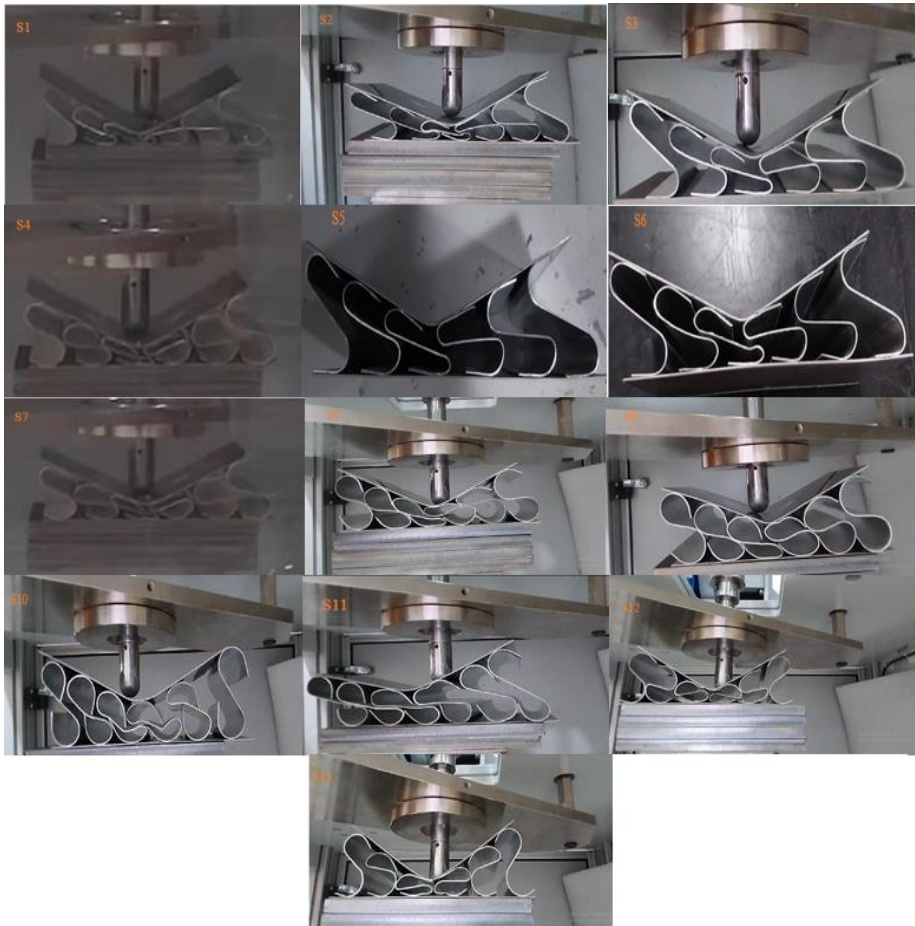
Figure 3. Low-velocity drop impact testing specimens[36]
