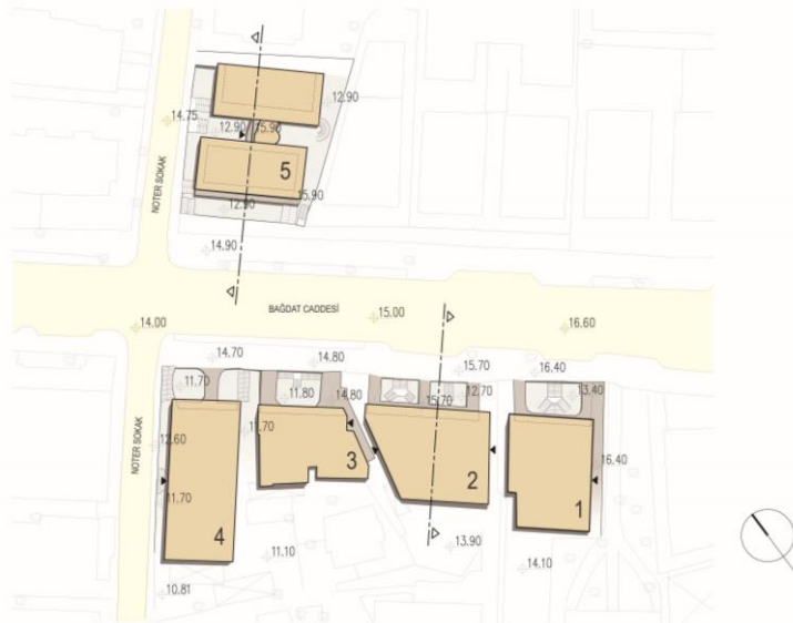
Figure 2. Plan of Buildings (aerial view) and the leveled retail spaces with the sunken courtyards. The black arrows indicate the entrances to the residential units (drawing by Gönül, 2024).
