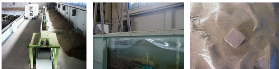
Figure 6. General view of the current channel where hydraulic tests were carried out (left), the wave being given in the channel (center) and the scours formed around the artificial reef block at the end of the test (right).
