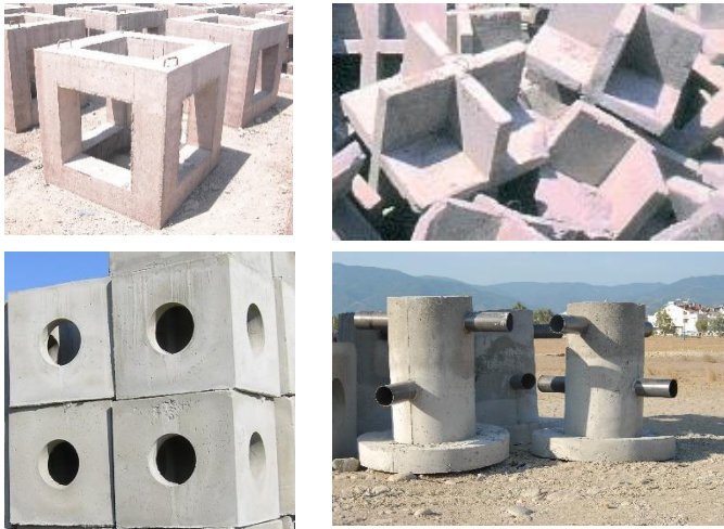
Figure 3. Artificial reef units of different designs constructed from concrete materials in Turkey.
