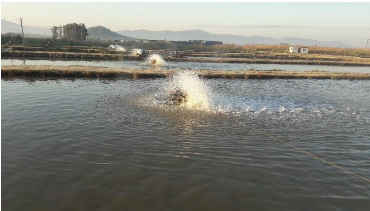
Figure 9. Pedall Wheel Aerators Using in Ponds
