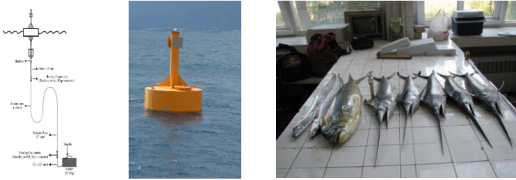
Figure 8. Technical drawing of the developed floating artificial reef (left), its surface view (center) and a sample of the individuals caught afterwards (right).
