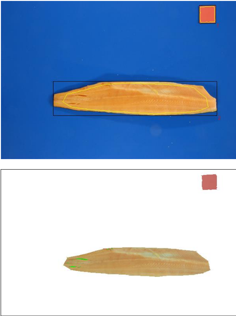
Figure 5. PSF number 6 (a) image before analysis of machine vision system, (b) image of PSF number 6 analysed by LensEye program
