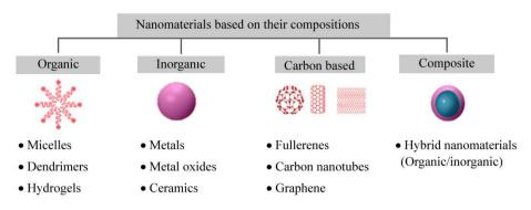
Figure 3. Classification of nanomaterials based on their compositions
