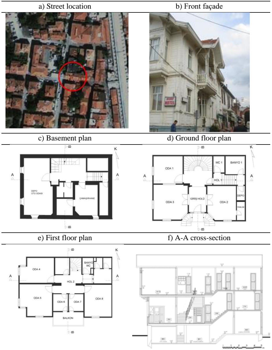
Figure 4. (a) Street location, (b) front façade, (c, d, e) floor plans, and (f) cross-section of the Aksaray Hotel (Building B)
