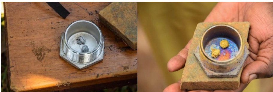
Figure 4. Appearance of amalgam before and after Hg removal in the distillation cell
