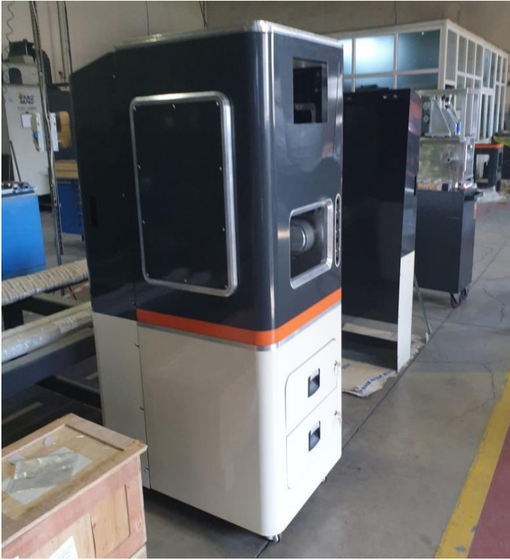
Figure 18: Automatic Control and Measurement Bench for Serial and Precise Measurement Control of Camshafts
