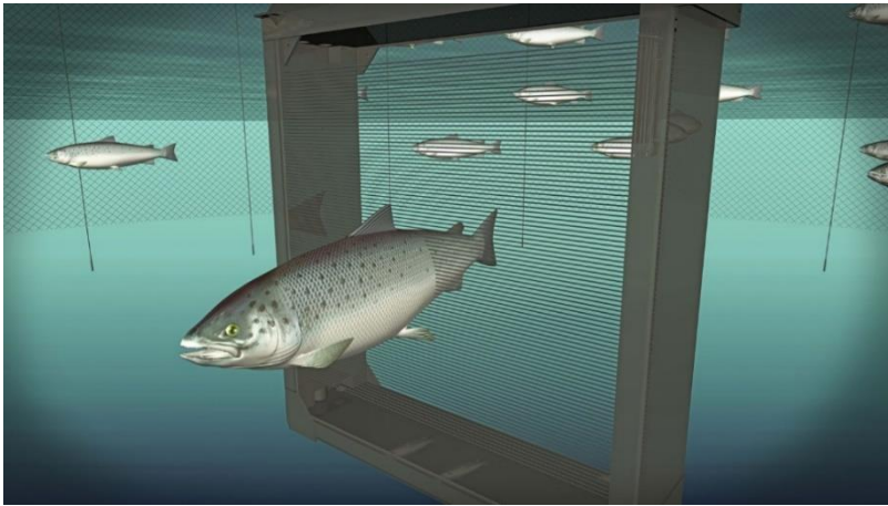
Figure.10. Consisting of a frame, this system provides a 24/7 overview of the average weight, size distribution, condition factors, and growth of fish within the cage (Anonymous, 2024a).
