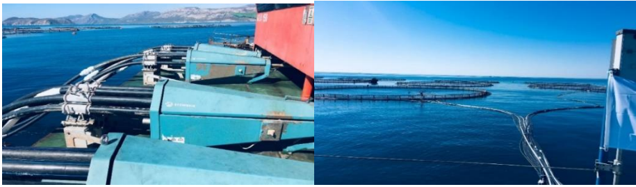
Figure. 5 Automatic feed distribution system from the feed storage unit (Barge) to the cages via pneumatic pipes used for feeding in offshore cage systems (Dikel 2023).
