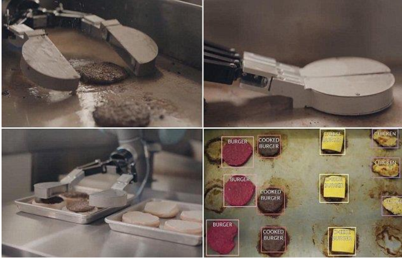
Figure 10. Flippy, the world's first autonomous robotic kitchen assistance by MISO
