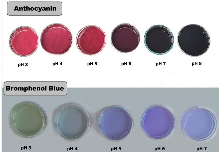
Figure 2. Color changes of anthocyanin and bromphenol blue in waters with different pH values.
