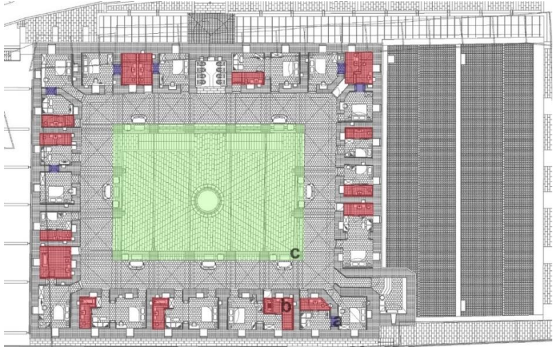
Figure 10. Deveciler Khan First Floor Plan, Restoration in 2019 (a) door openings b) wet spaces c) steel roof cover) (Tokat Regional Directorate of Foundations Archive)
