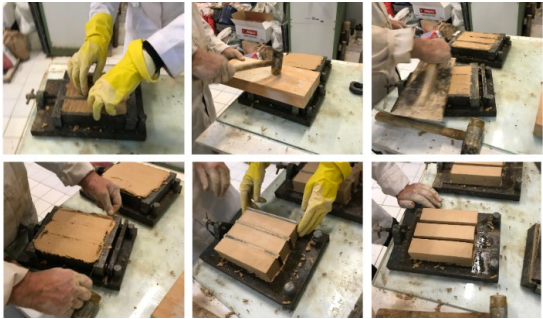
Figure 10. Moulding and demoulding process of samples (Created by the authors)
