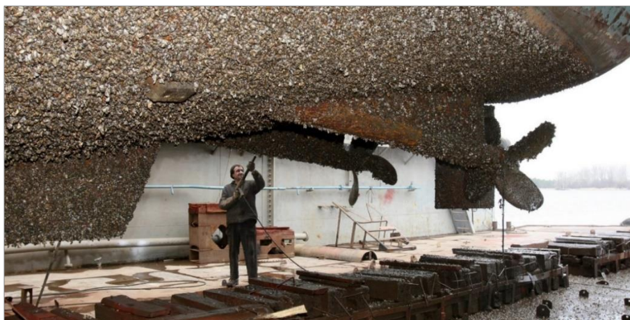
Figure 9. Heavily Biofouled Ship Hull
