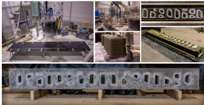
Figure 13. Beam Fabricated by Maitenaz et al. (2020).
