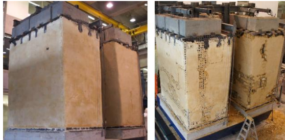
Figure 3. Strength Tests Performed on the Sample Placed on the Steel Mesh (Reyes et al., 2019).
