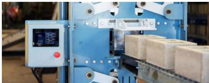
Figure 5. Soil Blocks Produced with an Extruder (Gelirli, 2022). Hydraulic press machines can be used in adobe brick production to achieve higher quality, smoother surfaces, and various designs(Figure 6). In a recent study, mud, fly ash, fibres, and aggregates were utilized, supplemented by additives and binders such as cement, liquid glass, and polypropylene fibers. These materials were added into the adobe in specific proportions, resulting in improvements in both compressive and flexural strength (Minh Trang, Dao Ho, & Babel, 2021).
