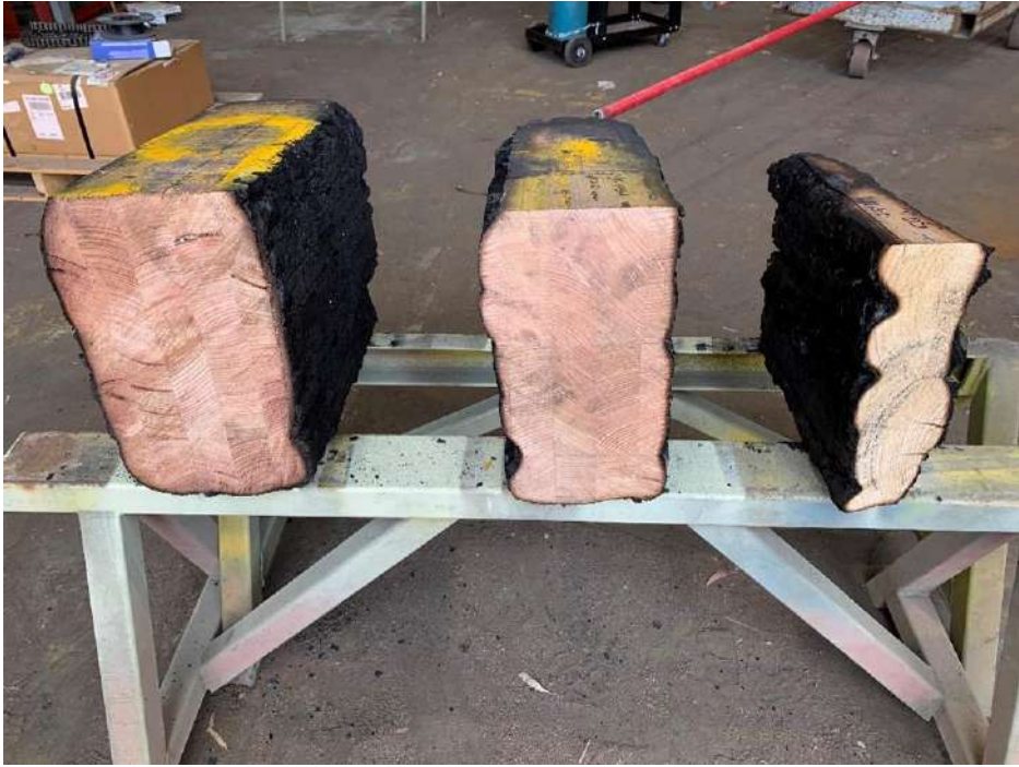
Figure 4. Grey Gum (Left), Tasmanian Oak/Victorian Ash (Middle) & Radiata Pine (Right) MASSLAM components after undergoing a 120 minute ‘loaded’ beam fire test.
