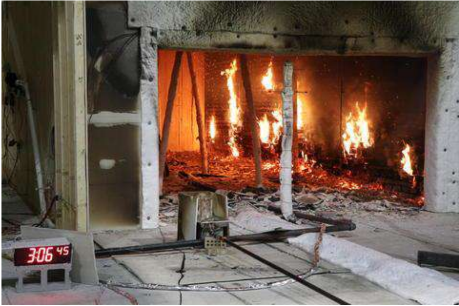
Figure 3. Mass Timber Fire Testing
