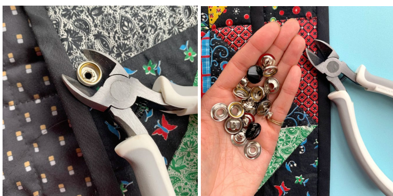
Figure 18. Manual removal of snap fasteners ( https://www.burieddiamond.com/blog/2021/6/29/how-to-remove-heavy-duty-snaps-tutorial-removing-dritz-heavy-duty-snaps )
