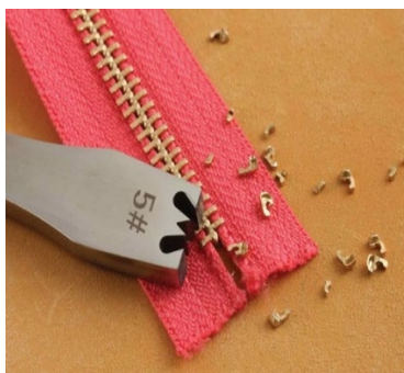
Figure 3. Manual zipper removal process ( https://craftingagreenworld.com/articles/reclaim-zippers-old-pairs-jeans/ , https://madeonjupiterleatherlab.com/products/zipper-teeth-remover?srltid=AfmBOorRKtDQsm5S22RFo_eg8iaT8EE37eIqV2zWzeQ0fLSNyLQDEQIz )
