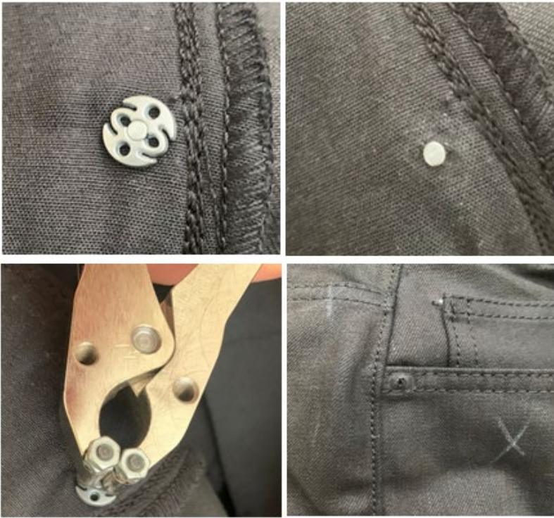
Figure 16. Removing the retaining component located beneath the rivet
